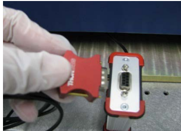
11. Connect 9 Pin Connector
