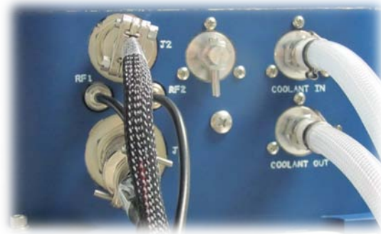
Figure 2-8 Laser Head Power Connection
