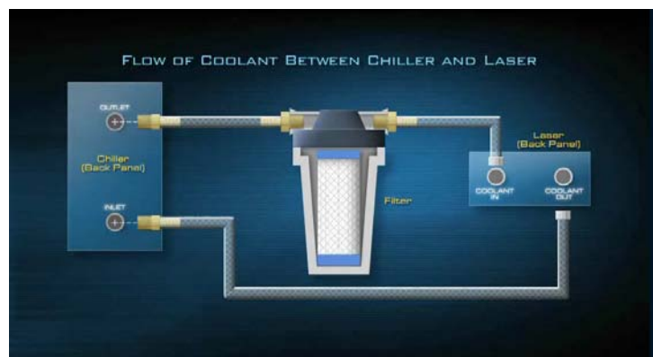
Figure 2-2 Diagram of Water Hoses and Filter Connections
