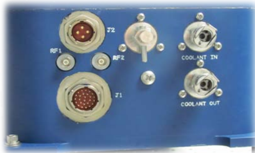
Figure 2-4 Connectors on the back panel of the Patara laser (Model Pa-100-QMG and PA-200-QMG).
