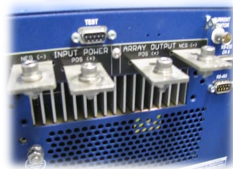
Figure 2-18 Input Power and Array Output Power
