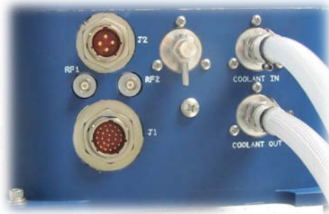
Figure 2-5 Laser Head Coolant Lines
