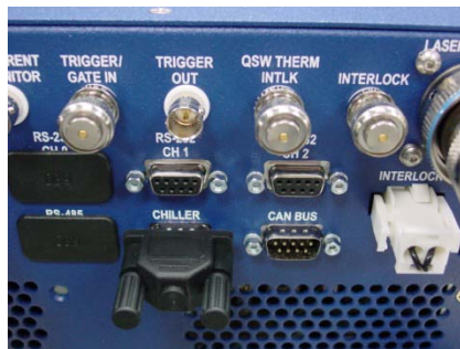
Figure 2-17 BNC Interlock Connection
