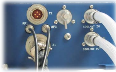
Figure 2-7 Laser Head RF Connection
